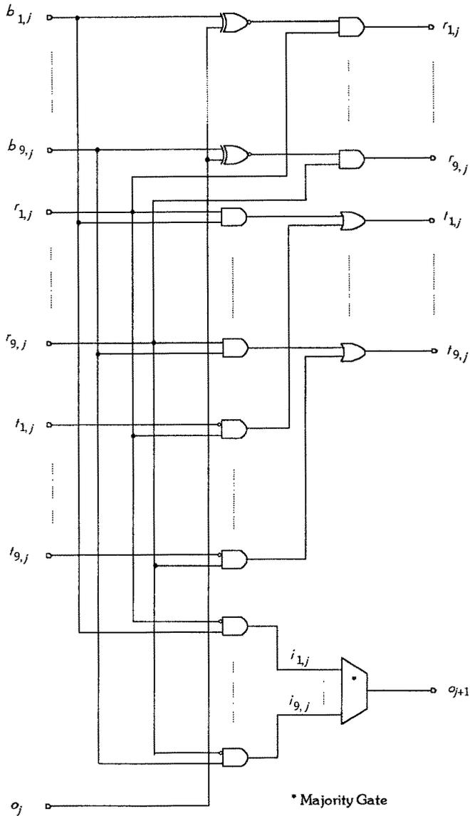
Fig. 4. The basic processing element (PE).
