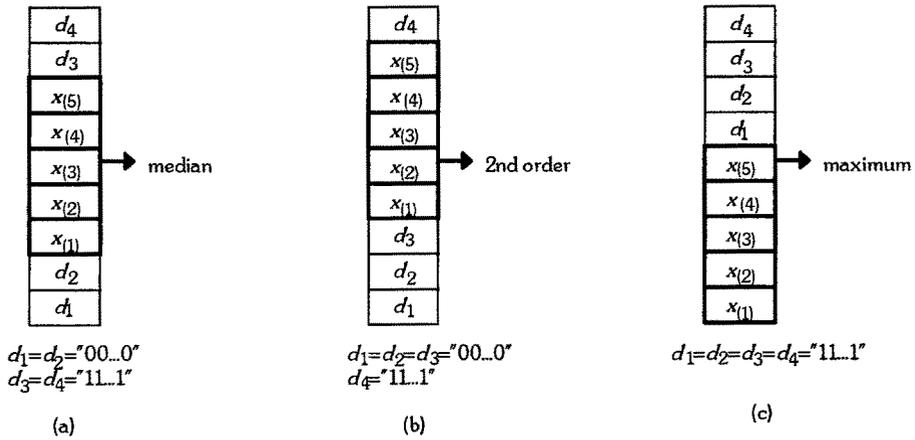
Fig. 1. Illustration of dummy inputs use : (a) median, (b) 2nd order and (c) maximum computation.
