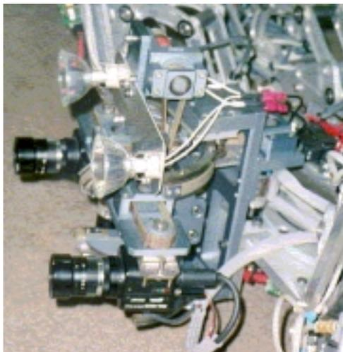
Figure 3: A close-up of the Eurohead mounted on the robot front.
