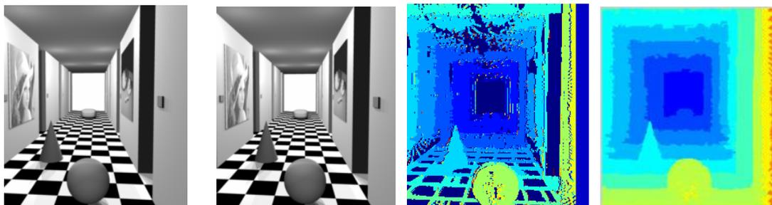
Fig 2. Left and right images. Disparity map before filtering. Resulting disparity map.
