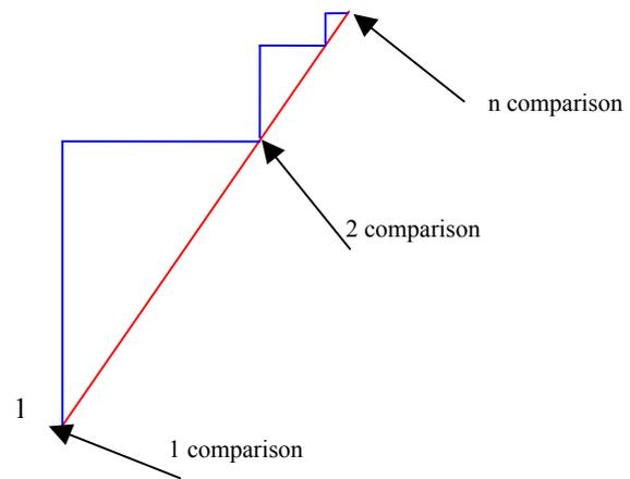
Figure 4: Successive approximation of the target with straight-line segments
