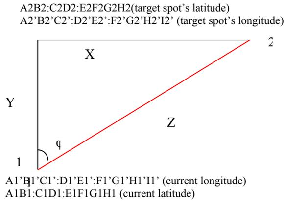
Figure 3: In order for the airplane to fly from waypoint (1) to waypoint (2), it has to cover a distance  $Y+X$  and not just  $Z$ .
