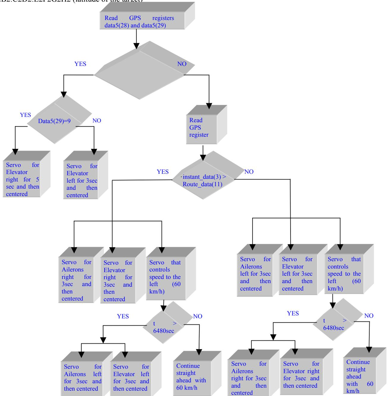
Figure 2: Decision diagram according to the signal from the GPS.
