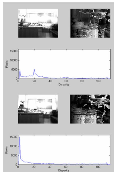
Fig. 5. Evaluation results for the case presented in Figure 2(c). On the upper side the fused images, the extracted disparity maps and the histograms of the disparity map are shown when the cameras are fully paralleled. On the lower side the same are shown for fully converged cameras. We can clearly notice that when the best vergence angle occurs, the majority of the disparities are close to zero.
