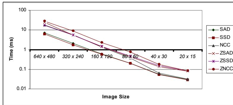
Fig. 4. Time performance for different image sizes and for each measure
