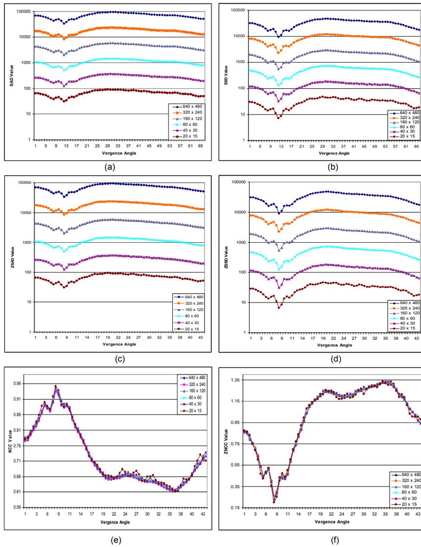
Fig. 2. Similarity indexes against the vergence angle for test image a. The lines correspond to the different dimensions. The minimum values represent the correct vergence angle except the NCC index where the maximum value corresponds to the highest correlation.
