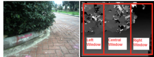
(a) (b) Figure 3. Reference image (a) and disparity map divided into three windows (b).
