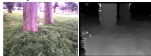
(a) (b) Figure 4. The reference image (a) and the produced disparity map (b).
