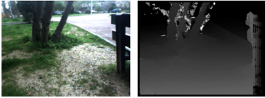
(a) (b) Figure 2. The reference image (a) and the produced disparity map (b) for a stereo pair.
