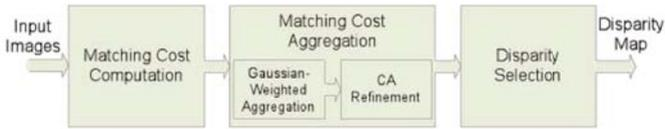
**Fig. 2.** Block Diagram of the Utilized Stereo Correspondence Algorithm
