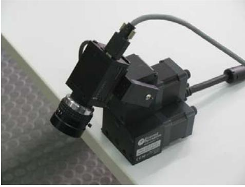
Fig. 3. The camera mounted onto a pan-tilt mechanism for the assessment of the vision system.
