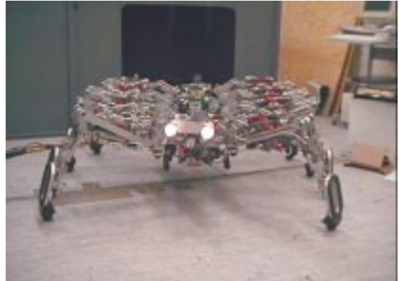
Fig. 1. The 8-legged pneumatic walking and climbing robot.
