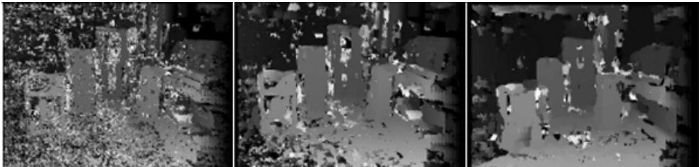
Figure 4. Detail preservation and noise occurrence in depth maps according to the value of the mask size (from left to right 1, 15, 25)
