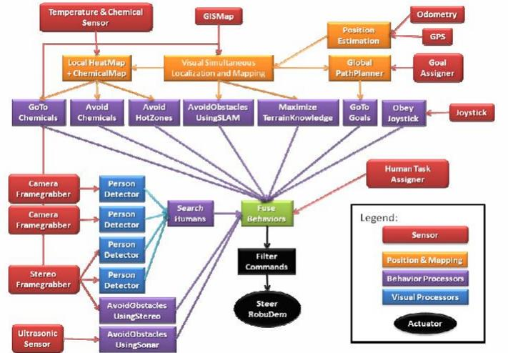
Fig.5. Behaviour based Navigation
