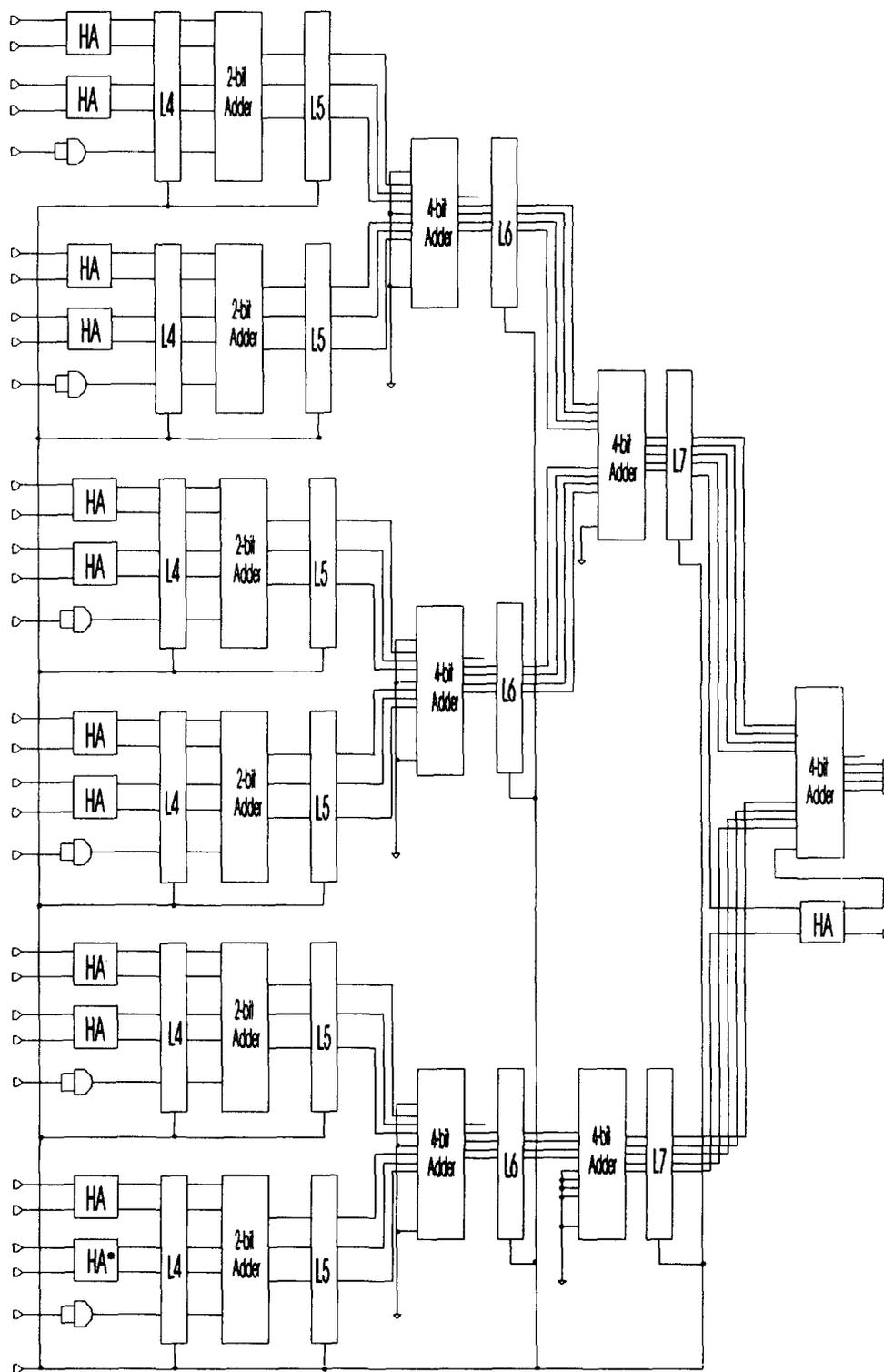
Fig. 5. Circuit diagram of the parallel/pipelined adder.
