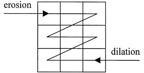
Fig. 3. Structuring element pixel loading in the cases of erosion and dilation.
