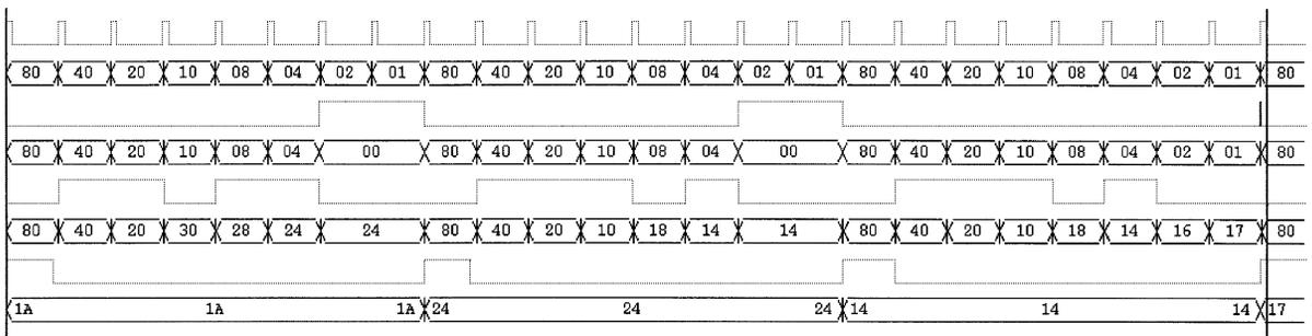
Fig. 7. Demonstration of the successive approximation technique.
