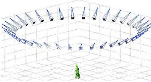
Fig. 2. Positions of cameras capturing a scene
