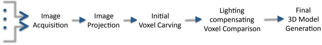
Fig. 1. Block diagram of the proposed method.
