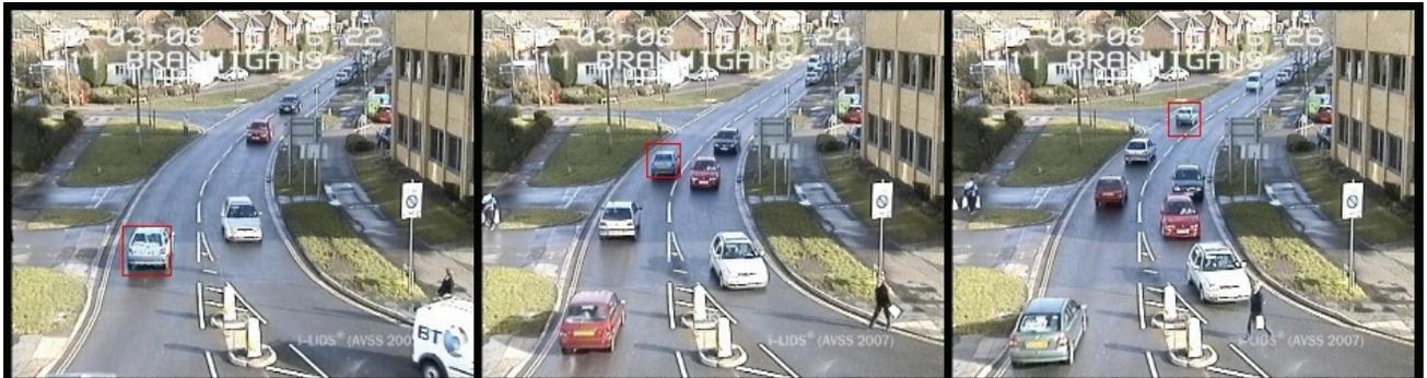
Fig. 5 Output of Moving camera subsystem in AVSS' scene. An object enters and exits in a shadowed region
