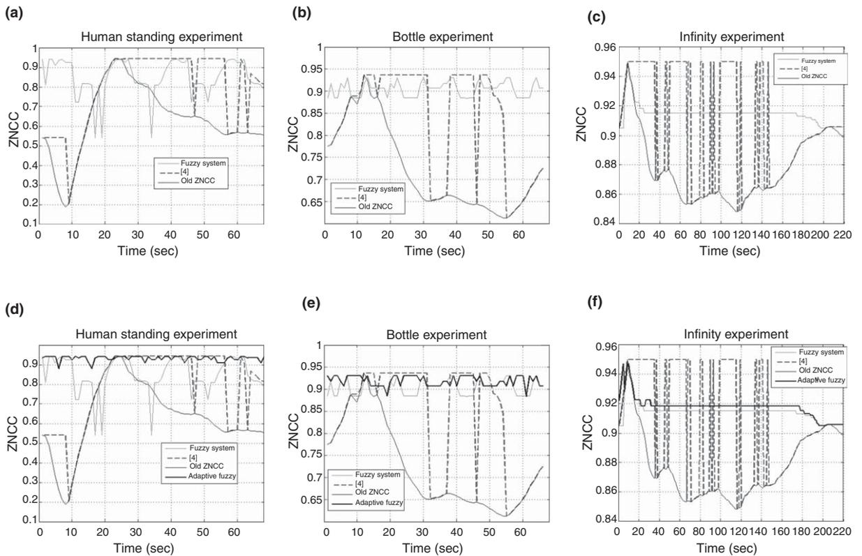
Fig. 7. The new ZNCC values acquired from the fuzzy system (gray thin lines) in relation with the old (black thin lines) and with the [4] ones (gray dashed lines) for the examined situations. The black bold lines represent the output of the adaptive fuzzy system.
