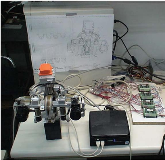
Fig. 5. The experimental setup: On the left-hand side the 4-d.o.f. robotic head; in the middle the dedicated PC for the image processing; on the right-hand side the four controllers for each of the d.o.f.; finally in the background the control PC.
