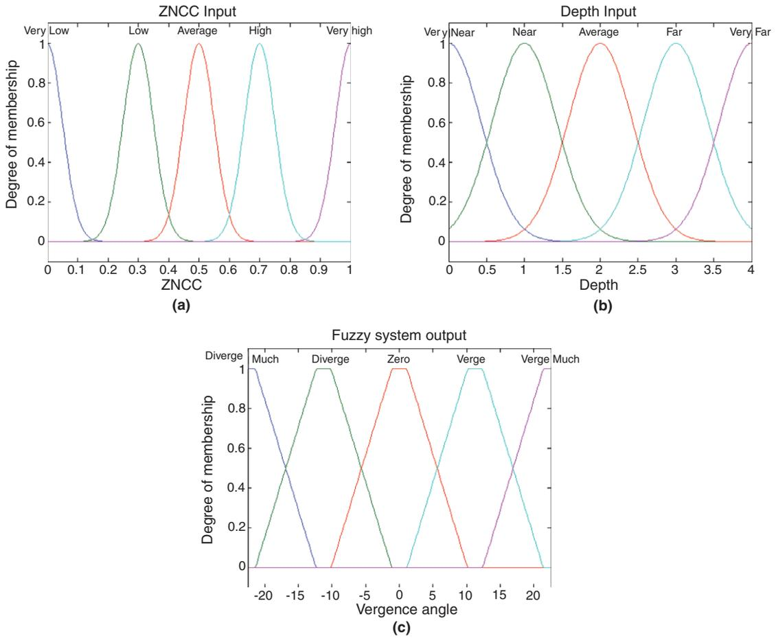
Fig. 3. Membership functions of the fuzzy vergence system for (a) input 1, (b) input 2 and (c) output.
