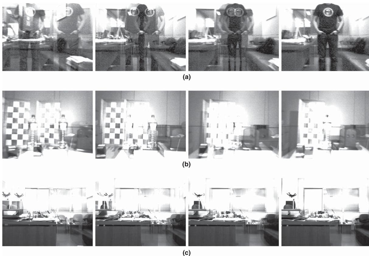
Fig. 6. Fused image sequences during the convergence of the system for several cases: (a) a human standing at a fixed position; (b) some objects were put in front of the robotic head and (c) there is absent of a specific target for the stereo vision system. From left to right, is displayed the index of the consequent vergence angles.
