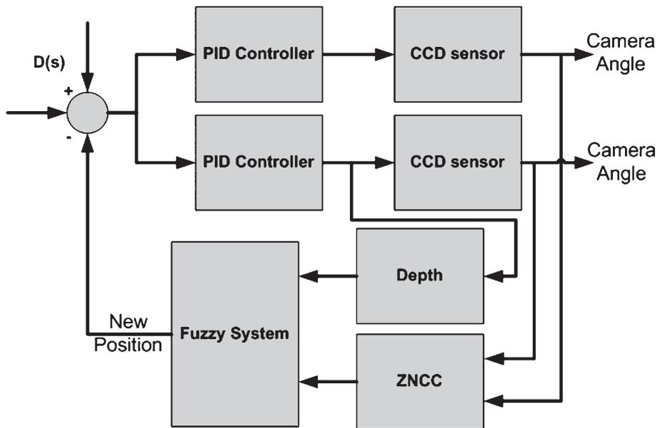
Fig. 2. Block diagram of the proposed automatic vergence system.
